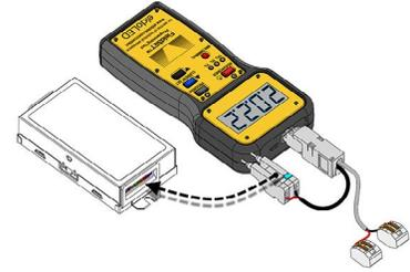
Once the desired settings are in the FieldSET Programmer Tool, settings are communicated to the replacement driver for installation!\*
